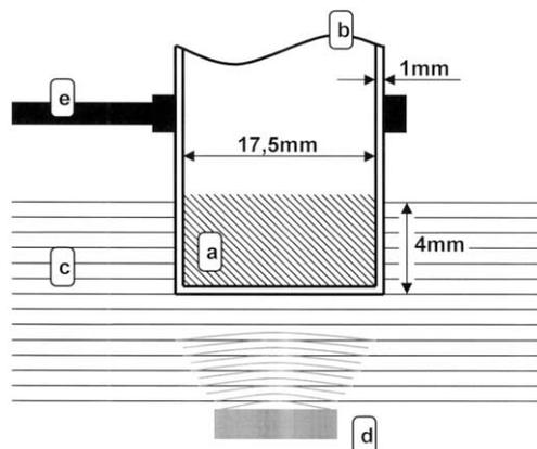
Fig. 1. Cross-section detail of the experimental setup. (a) Platelet-rich plasma sample (1 ml); (b) plastic test tube; (c) distilled water used to transfer ultrasonic waves emitted from the (d) ultrasound generator; (e) steel grips hold every test tube in reproducible position. Not drawn to scale.
