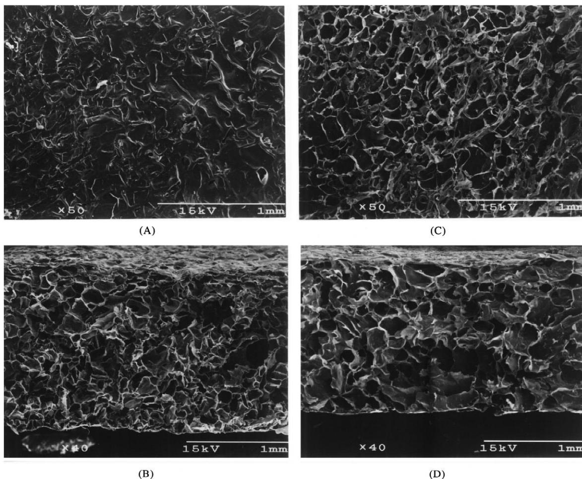
Fig. 1. Scanning electron micrograph of chitosan and CS–chitosan sponges. (A) Surface and (B) cross-section of chitosan sponge. (C) Surface and (D) cross-section of CS–chitosan sponge.
