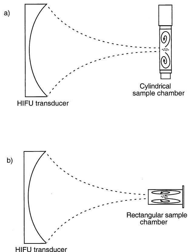
Fig. 2. Schematic of flow patterns in the sample chambers induced during CW HIFU exposures. For both types of sample chambers, the 1.1-MHz HIFU transducer focus is positioned in the center of the sample chamber. The general flow pattern is shown in (a) the rectangular sample chamber used in platelet adhesion studies, and (b) the cylindrical sample chamber used in activation and aggregation studies.
